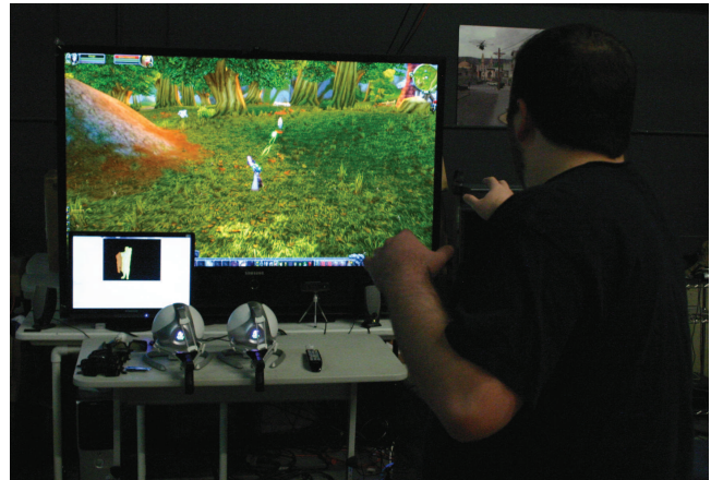
Figure 1: A user casting a spell using a “push” gesture in World of Warcraft, an off-the-shelf online video game that was not developed to support motion sensing devices. FAAST can be custom-configured to detect specific actions and bind them to virtual keyboard and mouse commands that are sent to the active window.
